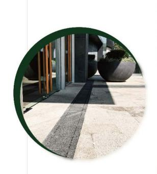
Casting Stone Grating is a precast unit fabricated using low content (about 15% by weight) of resin / polymer material as binder and quartz sand or crushed stone as aggregate, the mixed compound with designated color is filled into moulds and compacted to form panels to any shapes and architectural features through an advanced state of the art vacuum and compression process.
